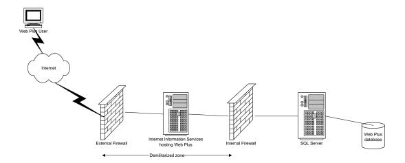
The security of Web Plus is based on the security of the client computer, the communication channel between the client and the web server, the web server, the base operating system, and the configurations of firewalls on either side of the web server. Use of strong logon passwords for logging in to Web Plus is utilized and the sharing of user accounts by users is prohibited.
